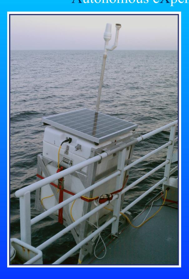
AXIS has been developed to provide the capability to deploy probes on a predefined schedule, or adaptively in response to specific events without the presence of an observer onboard.
